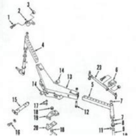
Fig. 3—Exploded view of straight adjustable front axle used on some tractors.
